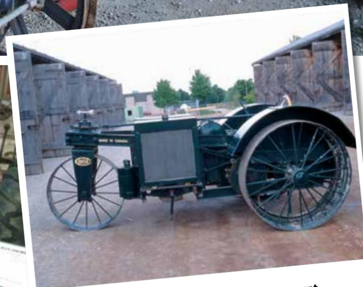
This Canadian-built Chase tractor has a crossmount engine and an unusual three-wheeled design.
