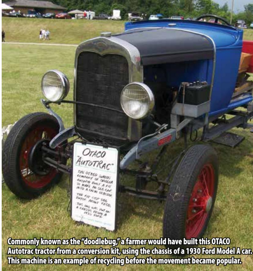
Commonly known as the "doodlebug," a farmer would have built this OTACO Autotrac tractor from a conversion kit, using the chassis of a 1930 Ford Model A car. This machine is an example of recycling before the movement became popular.
